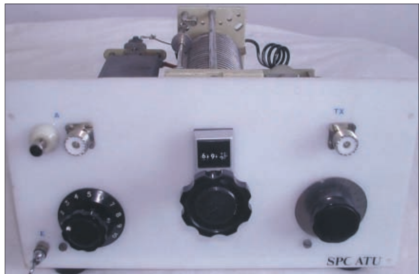
● Fig. 2: Front view of the a.t.u. which has a Perspex panel. The turns counter for the rotary inductor allows for quick band changing.
